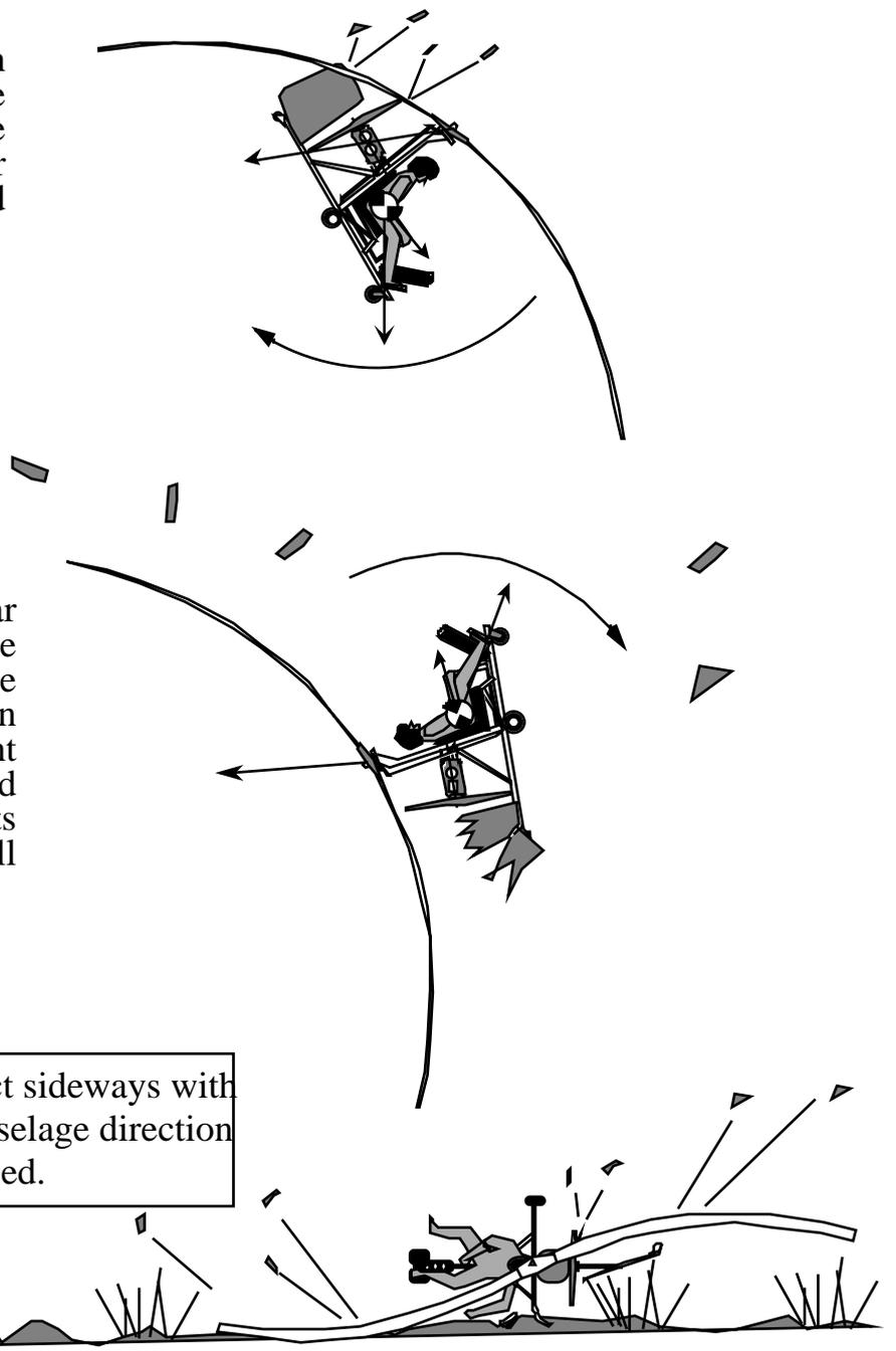
The eye witnesses were quite far and could not describe exactly the tumbling movements of the gyrocopter but in the final position the blades were highly bent upwards, a proof of low RPM and high velocity. Gyrocopter parts and pieces were scattered all around the place.
