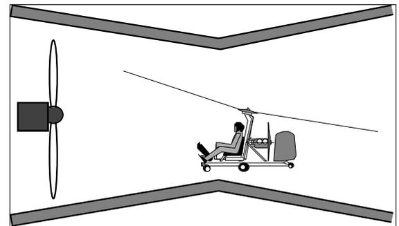
4. ...if no wind tunnels and funding are available for the purpose, test flight program with a radio controlled gyro-copter with and without a horizontal stabiliser (using a data logger and a chase plane to collect the data and make videotape of the gyrocopter response) or.....
