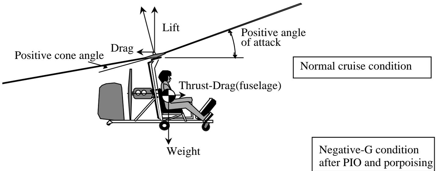
Negative angle of attack results in low RPM and large negative blade cone angle, rotor is hitting the flapping stops and finally rotor blades hit the vertical tail and propeller
